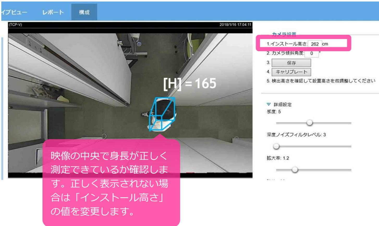
The screenshot displays the 'Camera settings' interface. At the top, there are tabs for 'ライブビュー' (Live View), 'レポート' (Report), and '構成' (Configuration). The main area is split into two sections. On the left, a live video feed shows a person standing in a room, with a blue bounding box around them and the text '[H] = 165' overlaid. On the right, the 'カメラ設置' (Camera Setup) section is highlighted with a pink box. It contains the following settings:
